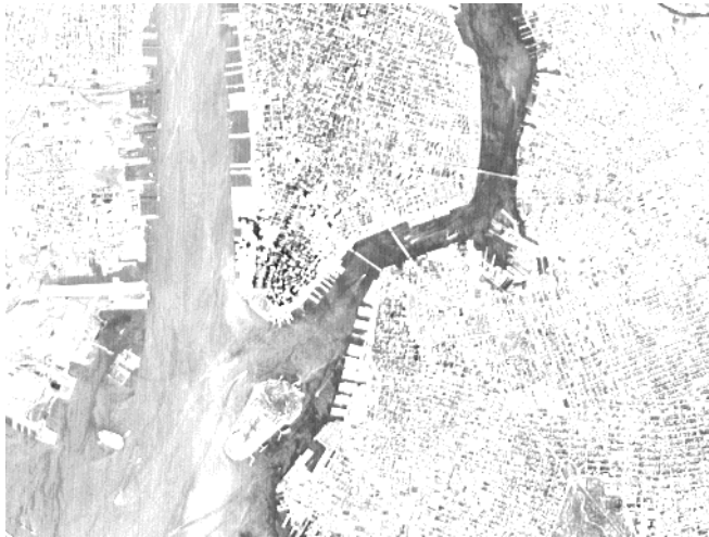
Figure 6-10: Image with Pixels <140 Scaled to Full Range of Brightness
