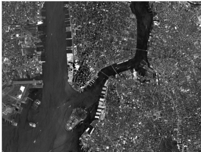
Figure 6-9: Image with Pixels >100 Scaled to Full Range Of Brightness
