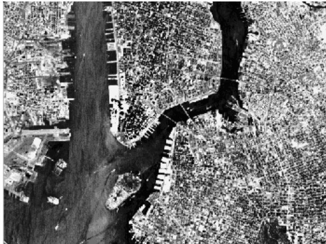
Figure 6-8: A histogram-equalized version of the image
